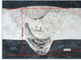
430F Stainless Steel Weld, Brightfield, Etched with Vilella's Reagent, 50x
