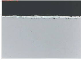
Water sensitive zinc coating, as-polished, 500x, Brightfield
