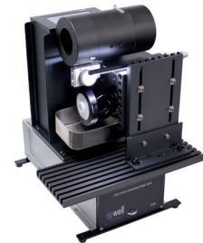
WELL 3500 Premium Diamond Wire Cutting System
